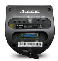
The Kick Type toggle\* sets the module to receive either a SWITCH signal or PAD signal from a kick trigger in order to play a sound.
